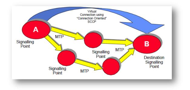
The solution to these problems was the creation of another protocol layer on top of MTP which was called the **Signalling Connection and Control Part (SCCP).** SCCP takes care of virtual connections and connectionless signalling.
